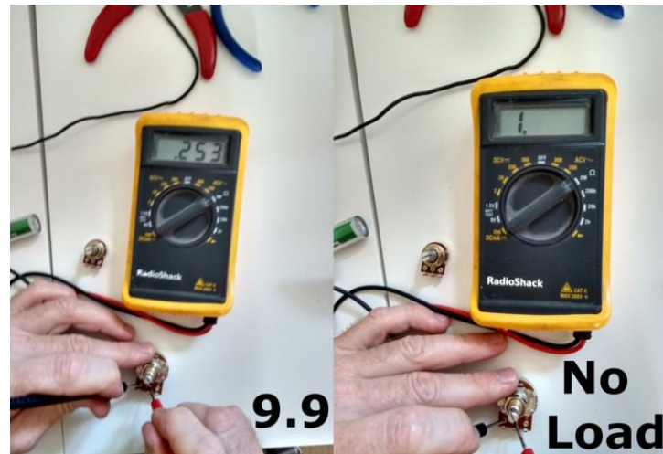
Figure 7 - new pot resistance
